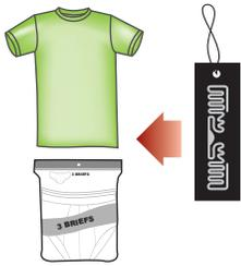
A. To poly bagged products with pressure sensitive stickers that incorporate the RFID inlays.
