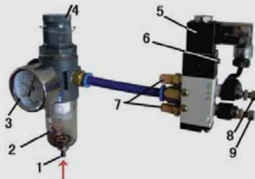
6. Manual button: Manual air supply (factory default setting. NOT recommended for readjustment).
